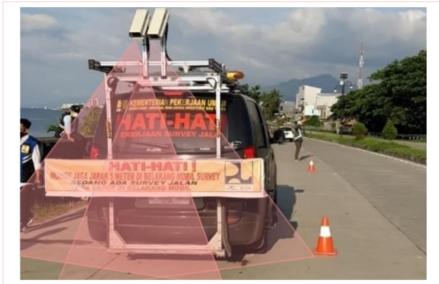
Figure 2. 'The Hawkeye' survey vehicle equipped with laser profilers, high speed cameras, a GPS, and a monitoring screen.
