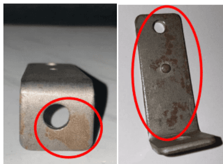
Figure 8. Rust on Stay L products
